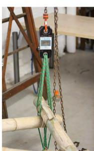
Triangle 3 (T3) 800x900x1000: twisted wire joint
