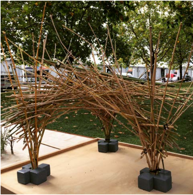
Figure 2: Scale models of structural bay of canopy (left) and pods (right) Images: Helen Norrie.
