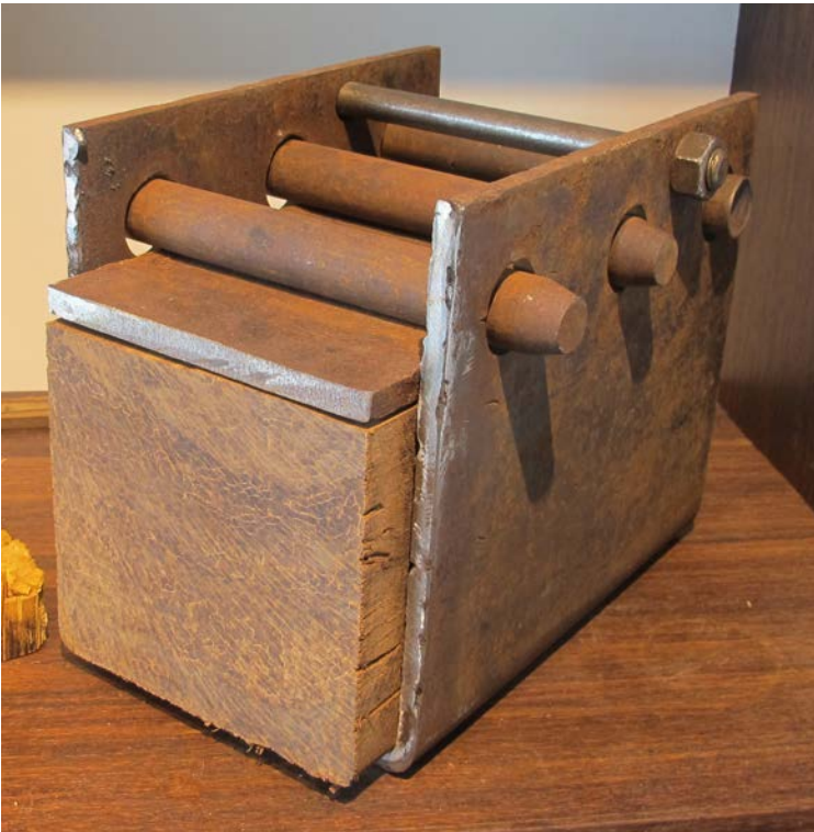
Sample of a cold press utilised in the manufacturing of bamboo laminate beams. Amsterdam, Netherlands
